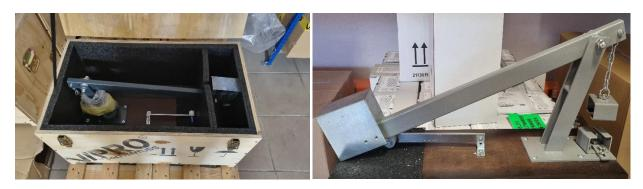
The "Weight" element has to be installed onto the "Working Arm" with a help of two screws (included).
