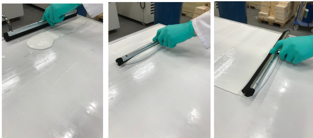
FIGURE 11 Application of flowable silicone sealant on a backsheet using a squeegee
