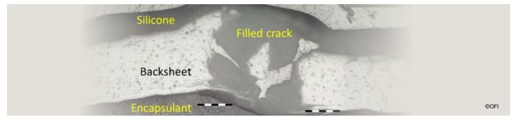
Tests were conducted at the Austrian Research Institute for Chemistry and Technology (OFI) and Silicon Austria Labs (SAL). It was shown that coating a module featuring deep cracks caused by degradation in the field, led to a restored insulation, that the module retained a high insulation after damp heat aging, and that it passed a subsequent wet leakage test.
