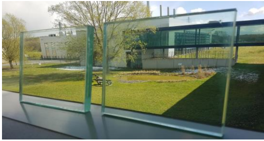
Figure 7: Glass-glass laminates with the two types of transparent edge structures, prior to damp heat ageing (right: laminate with only silicone hot melt edge material, left: laminate with combination transparent PIB and silicone hotmelt back-filling)
