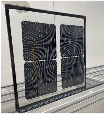
Figure 3: Photo of a four cells mini-module with TPS edge
