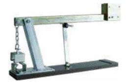
MANUAL TENSILE TESTER FOR H-PIECE SAMPLE is used in tensile testing of the structural silicone joint in structurally glazed façade elements. Measuring range: 42 kG breaking force - until the H-Piece sample ruptures.
