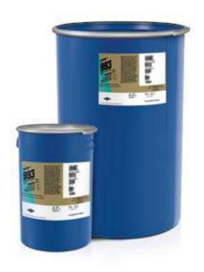
TWO-PART NEUTRAL CURING STRUCTURAL SILICONE SEALANT specialized sealant adhesive for the structural bonding of the glass onto the metal substructure of the curtain wall. Provides excellent adhesion to various construction materials including glass and metal (anodized and powder coated aluminum, stainless steel, etc.).
